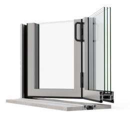
Separate environments and unify spaces with this bi-fold door system with an 80 mm deep frame. This evolution of the Bi-fold series offers an excellent thermal and acoustic performance, thanks to its 45 mm thermal break and a glazing capacity up to 48 mm.
