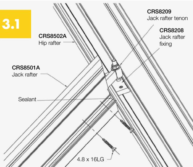
Locate the jack rafter tenon onto the jack rafter fixing bolt and adjust the lower nut to align gaskets, before tightening the the top nut. Then seal the jack rafter internally to the hip.
