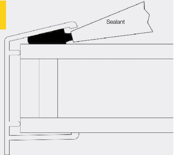
Fit the glazing end closures to the glass and run a bead of sealant between the profile and top pane of glass as shown above. **Only** use a suitable sealant with self cleaning glass. Soudal SMX 506 is recommended (available from Eurocell branches).
