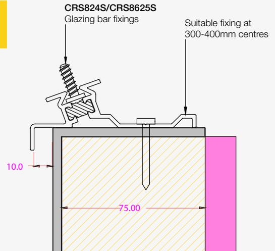
Ensure correct amount of glazing bar fixing studs are slid into the ring beam before any fixing commences. Position the ring beam so an equal overhang is achieved around perimeter and fix using suitable 5-6mm fixings at 300-400mm centres (starting and ending 100mm away from internal corner of the ring beam).
